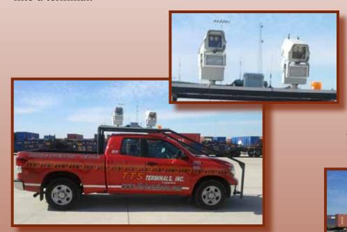
The Paceco® OCR system will read the container's ISO ID number from the front of the container when triggered by the container sensing system. The Paceco® OCR system has 90% or greater container reads. Cameras are configured to read both horizontal and vertical container
